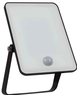
LEDVANCE floodlight with motion sensor - 20W - ESSENTIAL range - 1900lm - I P65 - 6500K
