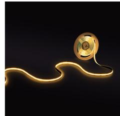
24V DC COB LED Strip - CCT - 14W/m - 10mm - IP20 - 5 meters roll - Cut every 26mm
