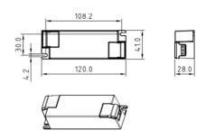
DALI dimmable DT8 CCT driver 220-240V - Output 6-54V DC - 250-700mA - 25 W
