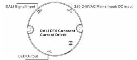
**Dimmable DALI driver - DT6 NFC single color 220-240V - Output 10-42V DC - 100-500 mA - 10W**
