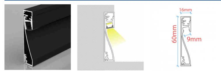
LED strip profile for skirting boards - 60x16mm - With diffuser - 2 meters
