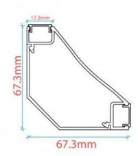
Double LED strip profile for corners - Surface - 67x67mm - With diffuser - 2 meters
