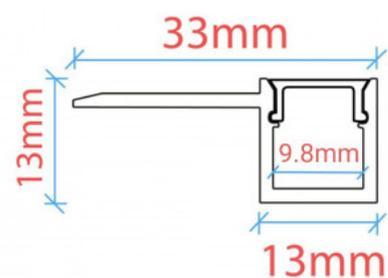
LED strip profile integration / trimless - One fin - 10x13mm - With diffuser - 2 meters
